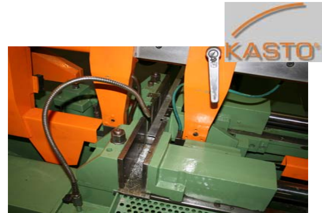
Endless saw Kasto SBA 220AU to 220mm bulk material Automatical feed & control of quantity
